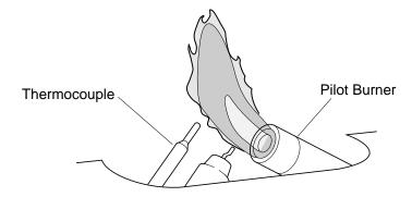
Figure 18 - Incorrect Pilot Flame Pattern
